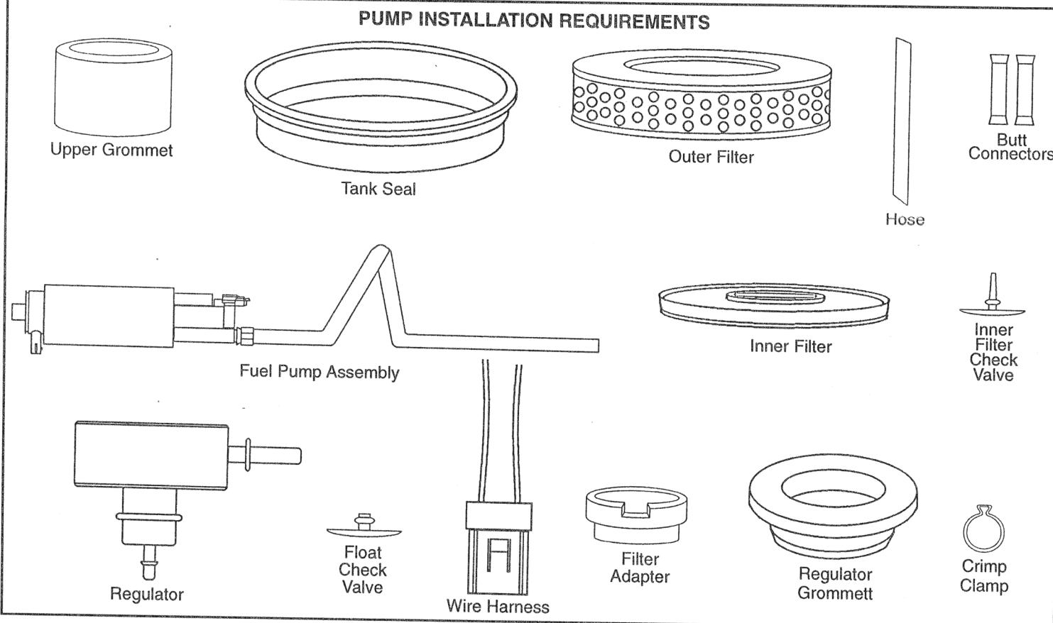
**WARNING:** This rotary fuel injection pump WILL NOT work on carbureted fuel systems. It is for electronic fuel injection only.
